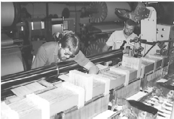
Weave Room Technician preparing a Sulzer Ruti weaving machine for style change.
