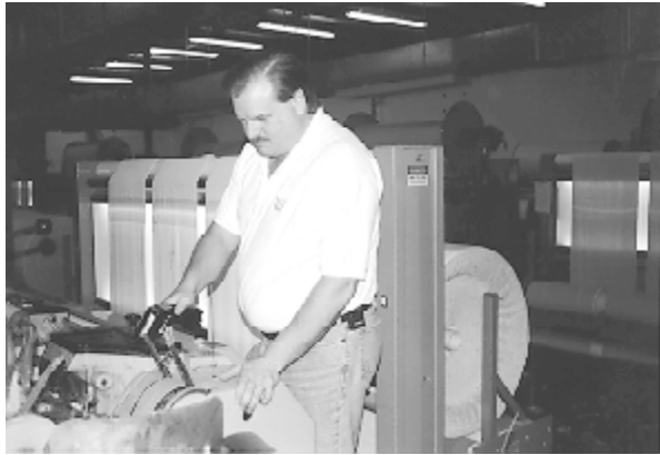
Chip Courtois, Weave Room Manager, taking temperatures of the lower picking house with an infrared temperature gun.
