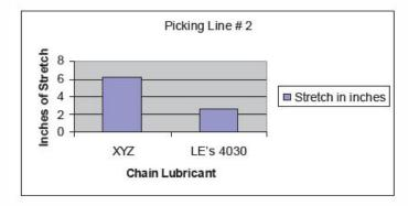
Estimated cost savings for using Quinplex 4030 in a 2-year period for all six chains used in plant, minus the cost of the lubricant is a net savings of \$96,000.
