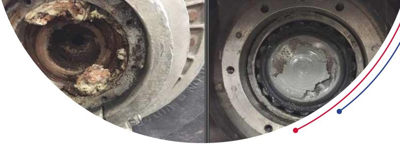
allowing the oil to run out of the thickener and bearing, while at the same time allowing the ingress of dirt and moisture. This led to complete saturation of the bearing and housing, which in turn caused excessive rust, lubricant degradation, bearing starvation, and numerous bearing failures.
