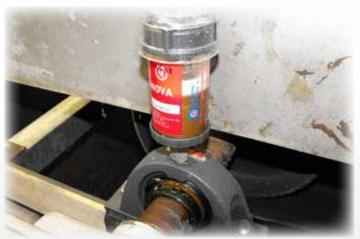
especially effective in severe operations caused by moisture or high temperatures. The lubricant's robust aluminum complex formulation seals out water and contamination and protects against oxidation, rust and corrosion. It also provides exceptional wear protection. Included in the formulation is Almasol, an LE proprietary additive which is a solid film additive that minimizes metal-to-metal contact further reducing heat, friction and wear.
