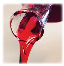
selection of hydraulic oil viscosity is critical to ensure satisfactory system performance. Selecting an oil with viscosity that is too low can lead to volumetric losses – bypass of oil around seals, pistons, vanes and gears. Selecting an oil with viscosity that is too high can lead to mechanical losses – sluggish controls, increased bulk oil temperature and cavitation. Both volumetric and mechanical losses contribute to overall performance loss in a hydraulic system.
