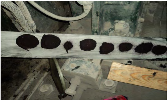
Figure 3. Before conversion to Pyroshield 9011: Spray nozzles blocked by excessive lubrication buildup affect the required intersecting spray pattern, causing an irregular spray pattern.
