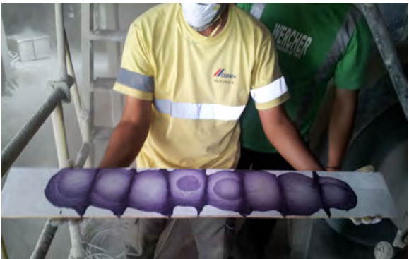
Figure 4. After conversion to Pyroshield 9011: No lubrication buildup on spray plate and no blockage on spray nozzles creates an equal distribution of lubricant.
