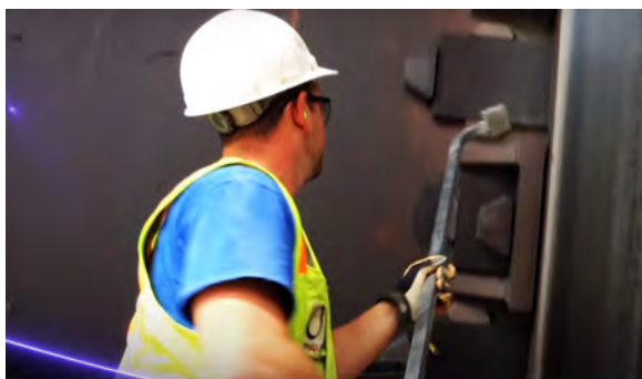
Figure 6. When placed between the tire bore and shell, the binder in the solid lubricant bar melts, and the kiln's rolling action distributes the lubricant where it is needed to protect the surfaces.
