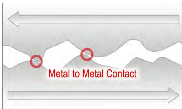
Figure 7. Asperities on touching metal surfaces.
