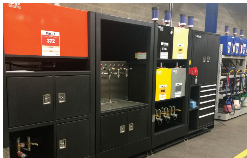
Figure 4: LE's new lubrication system keeps lubricants clean and dry with filtration into and out of each tank, and everything organized and color-coded for a smarter, more efficient process
