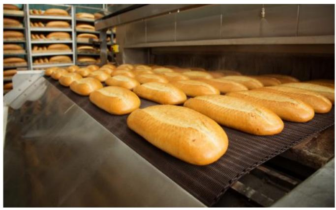
The high temperature environment in which industrial oven chains operate makes the choice of lubricant especially important
