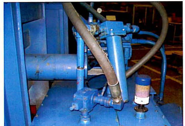
Figure 3. Breather Keeps Contamination and Water Out of System
