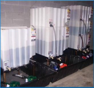
Tote-A-Lube storage tanks and Oil Safe transfer containers keep lubricants clean and contaminant-free
