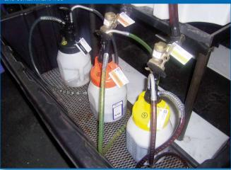
bottles used to transport oil to the units were exposing the oil to contamination. These open and unlabeled containers were also leading to oil mixing, which caused early drain intervals and other problems.
