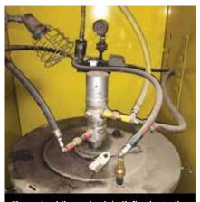
Figure 4: adding a check (relief) valve to the spray system (back of photo) saves Lehigh Hanson thousands of dollars
