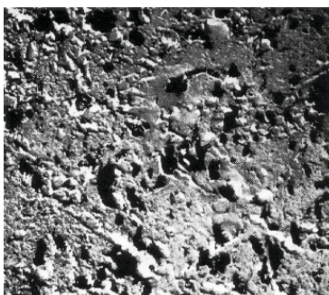
Figure 3: Photomicrograph of piston skirt lubricated with commercial oil, showing wear rate of 3.5 mg per hour
